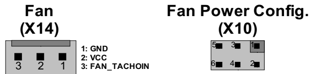
Figure 4-7. X14 Fan Connector and X10 Fan Power Jumper Header
